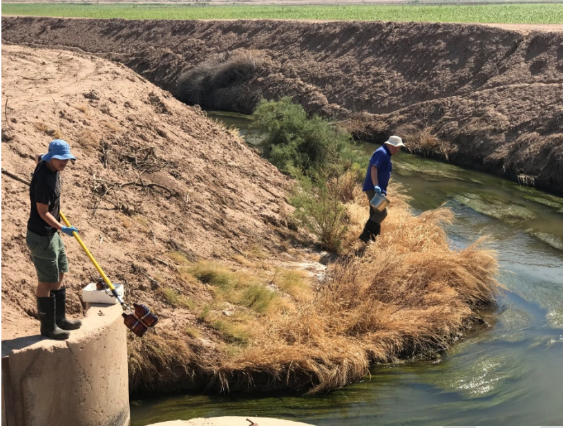
Photo Caption: DPR Environmental Scientist Anson Main and Scientific Aide Mason Zoerner collecting water and sediment samples at Rice Drain 3, Imperial. DPR analyzes the water samples for pesticides. Photo Credit: Xin Deng.
