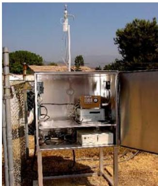
Ultrafine Particle Sampler
