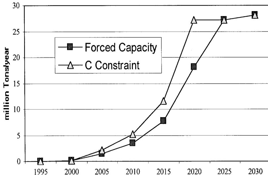
Figure 4. Carbon emissions displaced by PV in US-NE
