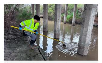
Scientific-Aid Tou Vang conducting surface water sampling at an established site (Imp\_Holtville) in Imperial County as part of the Southern California agricultural monitoring study. Samples were analyzed to assess short-term changes and long-term trends of pesticide concentrations in surface water resulting from agricultural runoff and their potential impact to the surrounding aquatic environments.
