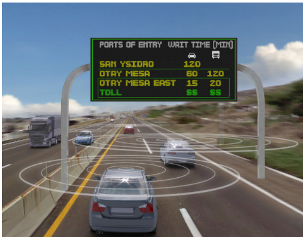
Caltrans/SANDAG simulation of the Border Wait Time System
