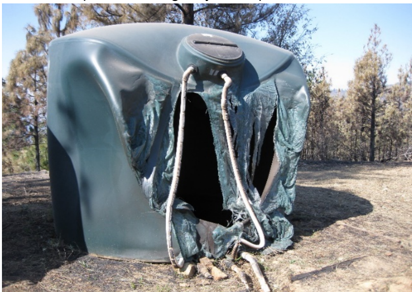
A tank used to store drinking water that was destroyed during the North Complex fires. Photo provided by Reese Crenshaw, State Water Board.
