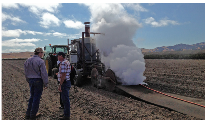
DPR funded research on fumigant alternatives using steam as an alternative to injecting chemicals into the ground to control soil-borne pests and diseases
