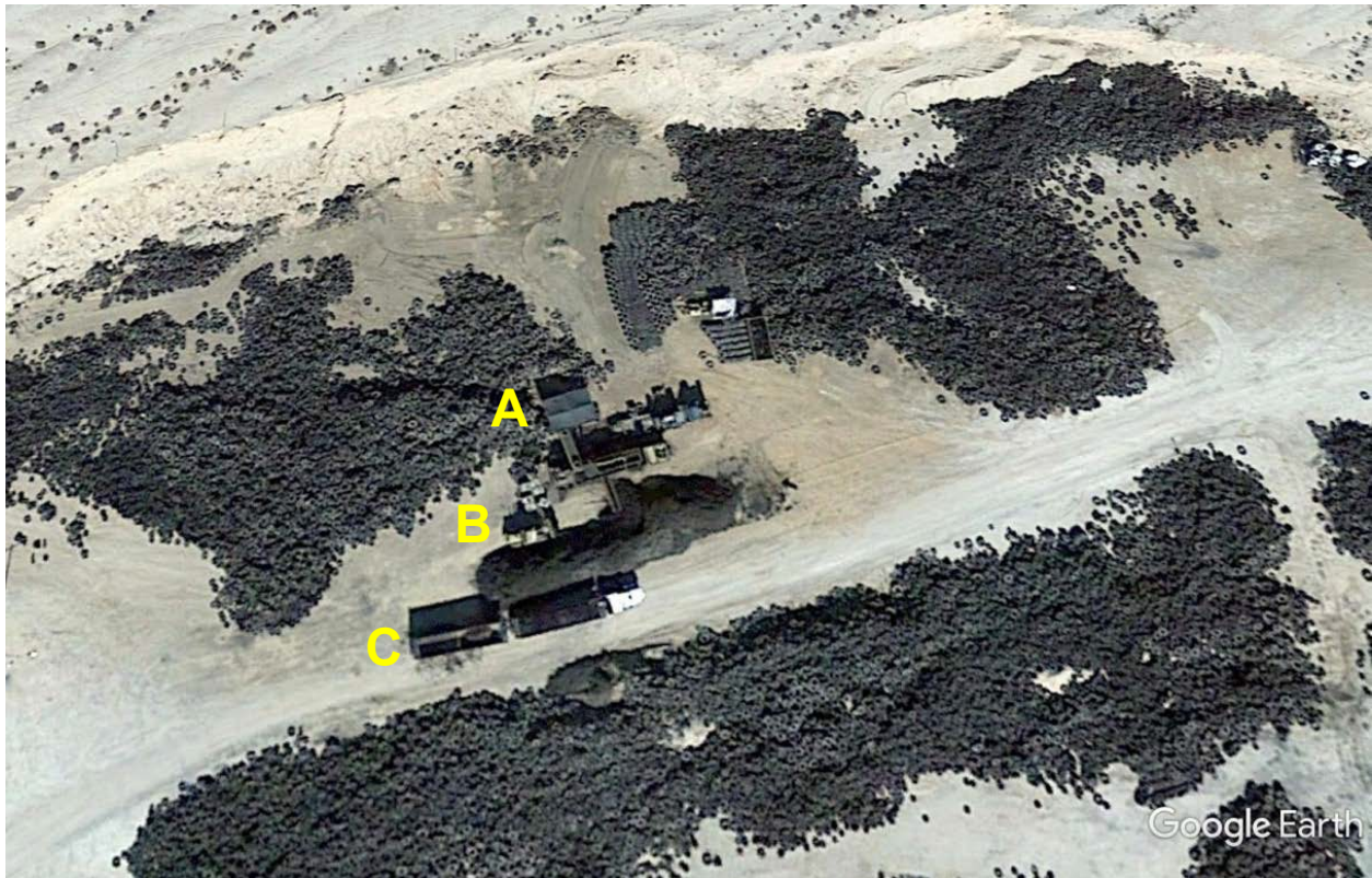
Image 8. Satellite image of CATENED I (Mexicali). Note the shredding equipment (A) and the front-end loader (B) filling the trailer (C) with shredded tires for transport to the Hermosillo cement kiln. November 2016. Source: GoogleEarth.
