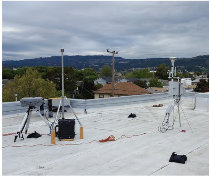
This is a DRUM sampler that was placed on a roof in East Oakland to monitor for particulate matter.
